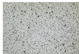
Ag/ZnO 92/8 SPW cross section
