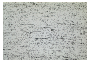
Ag/ZnO 92/8 SPW longitudinal section
